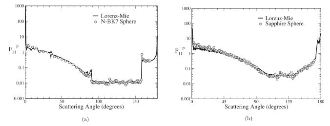
Figure 2. Comparison of phase functions based on the measured data and the Lorenz–Mie computations (solid black) for the N-BK7 (a) and Sapphire (b) calibration spheres (gray circles).
