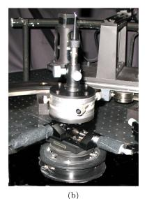
Figure 1. (a) Schematic overview of the experimental light scattering apparatus as seen from above. (b) Photograph of the flat black holder mounted on the x-y rotating table. The N-BK7 glass sphere is located on its conical tip.
