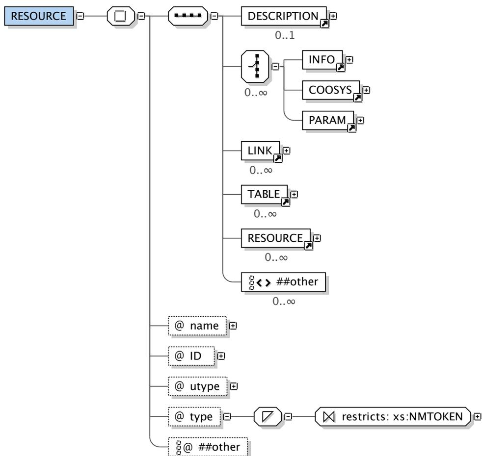
Figure C.3: Elements of the `<RESOURCE>` tag. `<RESOURCE>` tags can contain many of the tags the `<VOTABLE>` tag can hold, but additionally it can contain `<LINK>`, `<TABLE>` and `<RESOURCE>` tags. `<TABLE>` tags are used to include tabular data, while `<LINK>` tags are used to point to non-tabular data resources being described by `<DESCRIPTION>`. Generated with the XML Schema diagram generator of the oXygen XML Editor.
