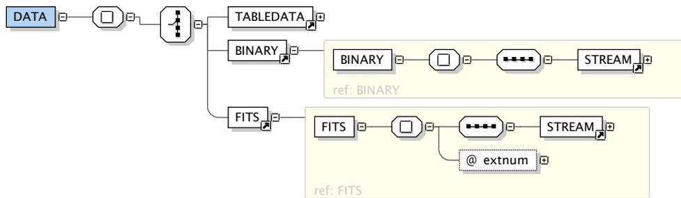
Figure C.5: Elements of the `<DATA>` tag. In a `<RESOURCE>` tag, tabular information is included within a `<DATA>` tag. That information can be pure XML tabular data within a `<TABLEDATA>` tag, a linked FITS file within a `<FITS>` tag, or embedded binary data within `<BINARY>` tag. The `<STREAM>` tag contains either the data or references to the data. See figure C.7 for more information. Generated with the XML Schema diagram generator of the oXygen XML Editor.
