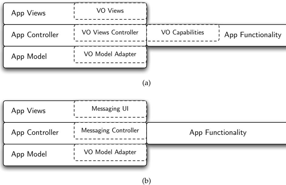
Figure 10.1: Comparison between the functionality to be added and/or modified in a VO-enabled application, both for a monolithic approach (a), and for a messaging-based approach (b).
