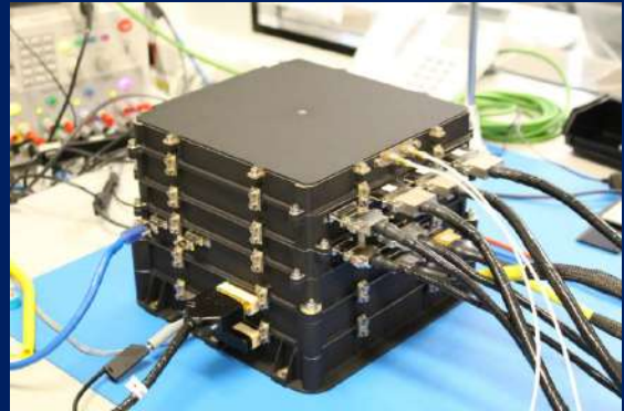
Qualification model for the SO/PHI electronics unit
