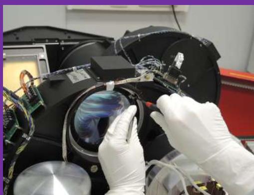
Installing new Br-gamma filter in PANIC
