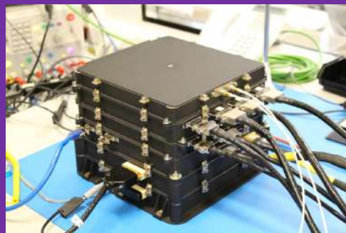
Qualification model for the SO/PHI electronics unit
