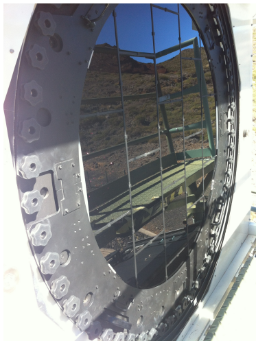
Figure 2.19: Filter for moonlight observations.
